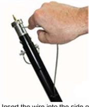
Insert the wire into the side of the slot and through the hole in the I-LAG™ screw. Then bend the wire end down.
